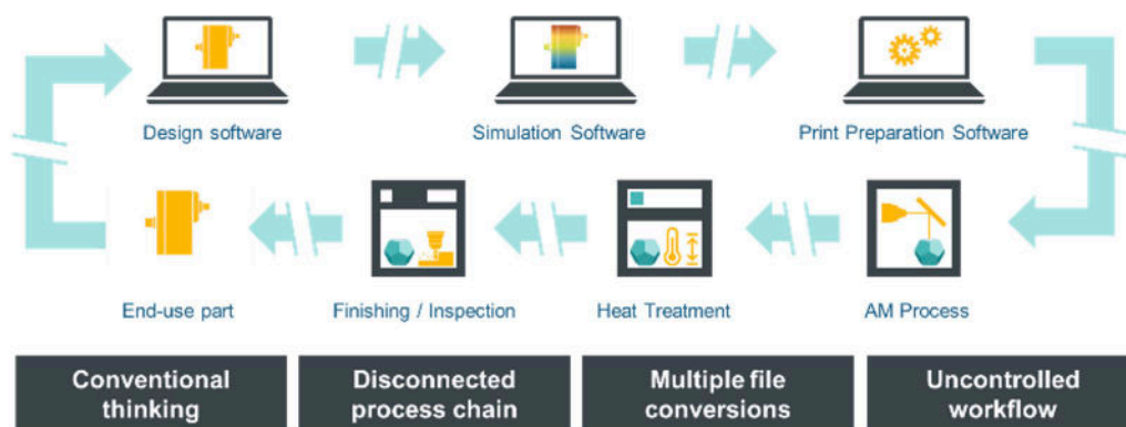
Figure 4. The normal disconnected AM software process.
