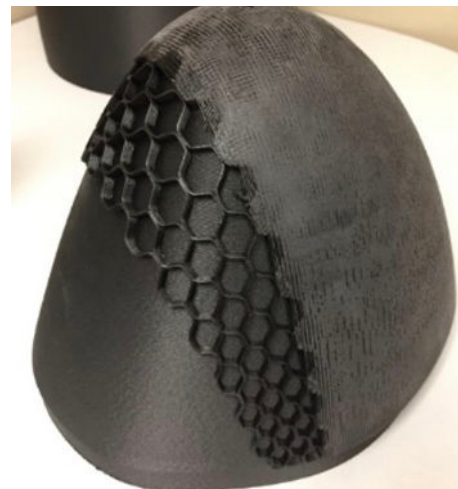
Figure 8. NX equips users with body lattice applications to design for additive manufacturing.
