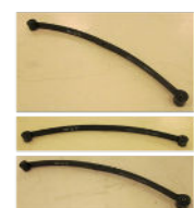
3 sets of rear leaf spring (vertical stiffness) with bushings
